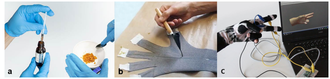
Figure 5: (a) polymerization chemistry (b) a glove before functionalization (c) the glove used in a 3d application.
