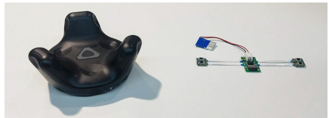
Figure 6: The HTC Vive Tracker and the HiveTracker, my open source reverse-engineered version.
