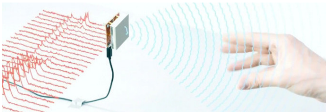
Figure 4: Google Soli visualization of its radar operation.
