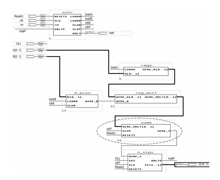
Other delicate point, before arriving in input of summ, this sequence of vectors has to pass by the register A (regA) and to be multiplied by the LSB of the regiser B (b\_piso) !!!
