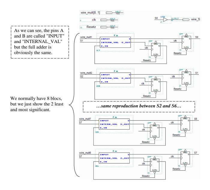
The test becomes really harder because C\_out is fed back in the C\_in (with a D flip flop on the way) and S is injected in the next full adder (also with a D flip flop on its way!)
