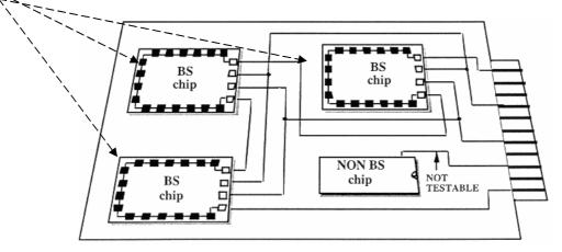
The BST circuits contained on a board are then connected together to form a single path through the board (require less I/O that my previous idea, but it's more complex to use). The boundary scan path is provided with serial input and output pads and appropriate clock pads which make it possible to:
